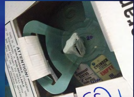
Seal Cylinder valve after testing
